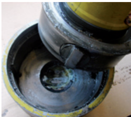
Check the quantity of grease in the clutch
