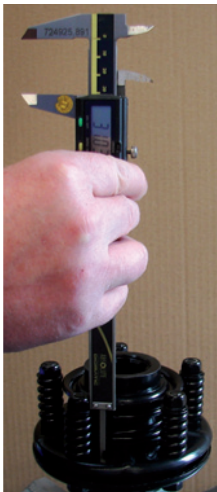
Measure the compression of the springs before removal so they can be set properly again afterwards
