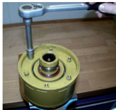
Release the tension from the plate type clutch after a longer period of disuse and remove any caked on residue
