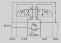
Saturn electric control valves with base plate, with part numbers that start with SKLS031C..., come in 12 and 24 volt models and can be supplied with a closed middle position (A and B closed, P and T connected) or a fully open middle position (A, B, P and T connected).
