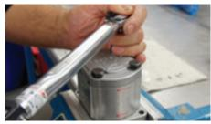
**12.** Install the bolts and tighten them to 45 Nm (aluminium cover) or 70 Nm (cast iron).
