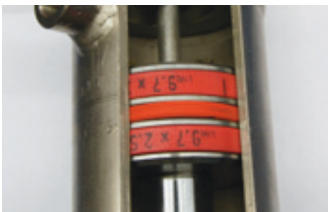
Using electromagnetic position determination, a cylinder equipped with a measurement system can indicate its exact length setting
