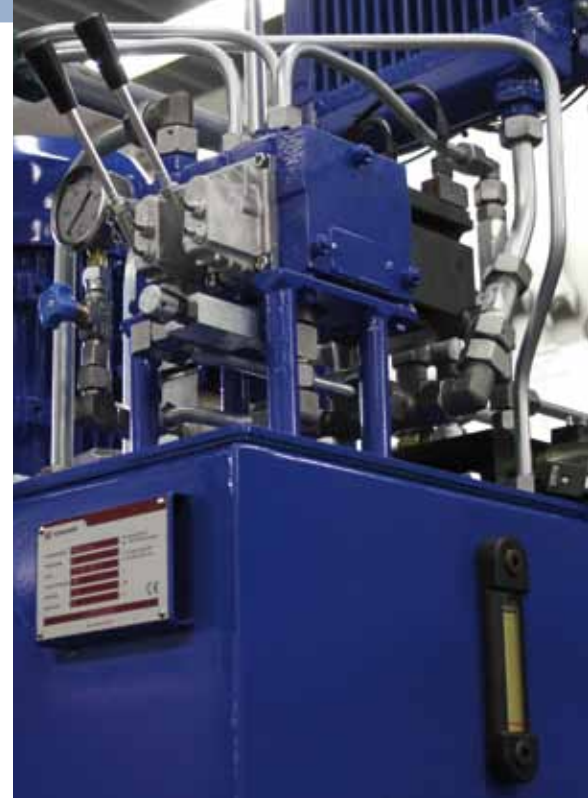
↑ The test stand produced in KSC can withstand a static load of up to 43 tonnes.
