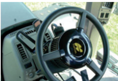
AES-25 Electric Steering automatically keeps the tractor on the right track.
