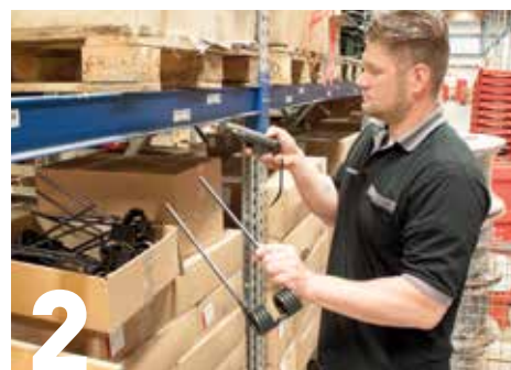
The order picker sees the exact quantity and the location of the rack on the screen of his hand scanner.
